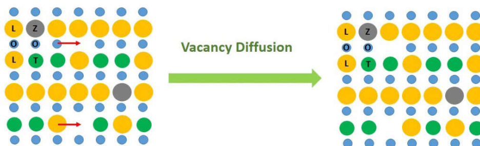
Fig. 2. Schematic representation of vacancy diffusion mechanism after addition of ZnO
