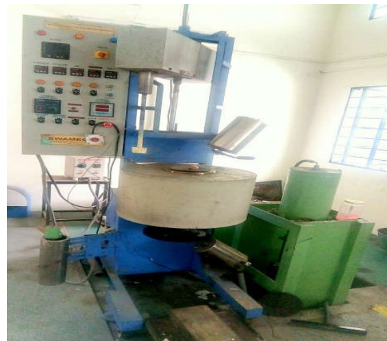
Fig. 1. Squeeze casting machine setup
