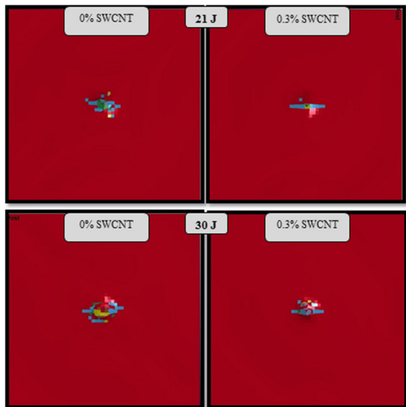
Fig. 10. Comparative LS DYNA simulation images of back-face damage for pure and incorporated GFRP with 0.3 wt% of SWCNT subjected to 21 and 30J energy.
