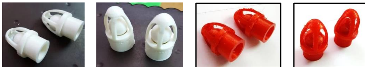
Fig. 6. The 3D printing of an artificial conical caged ball heart valves.
