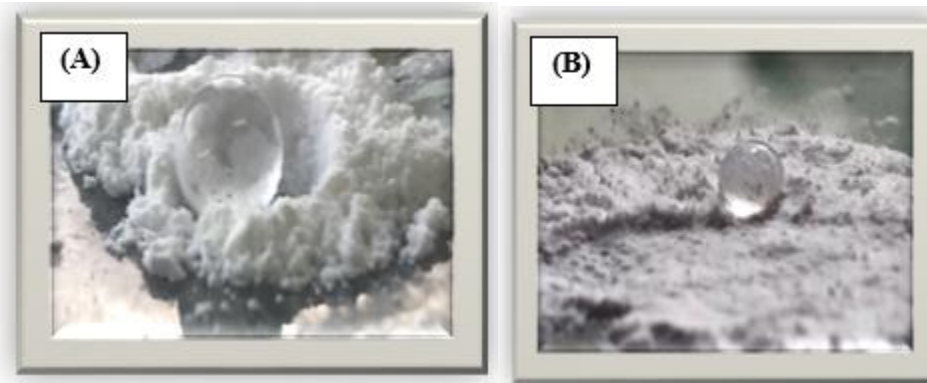
Fig. 3. The nano-silica powders hydrophobized by (A) ODTs and (B) HMDS
