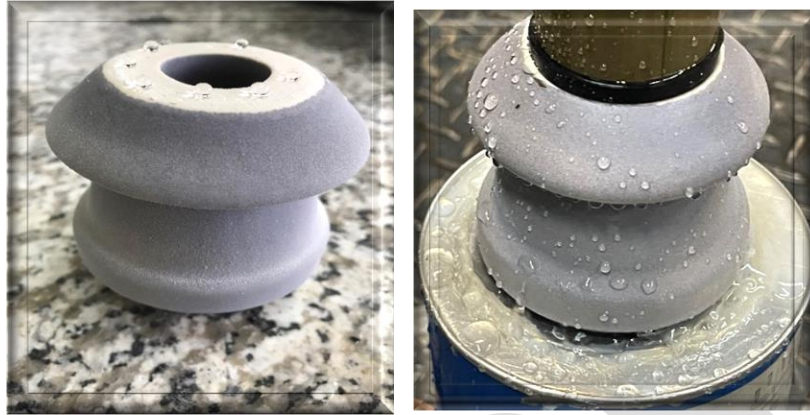
Fig. 5. The coated insulator after water spray
