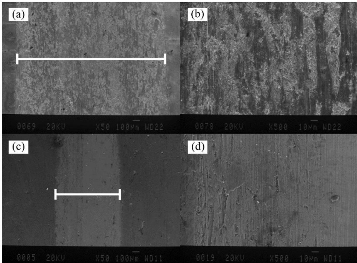
**Fig. 6.** SEM images of (a) H13 sample wear path  $\times 50$ , (b) H13 steel wear path  $\times 500$ , (c) CrN/AlCrN multilayer coating wear path  $\times 50$ , (d) CrN/AlCrN multilayer coating wear path  $\times 500$ .
